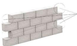
At this point masons needs to cut the full size block to half/quarter to fill the gap which may occur in the column wall juntion or between new wall to old wall.
